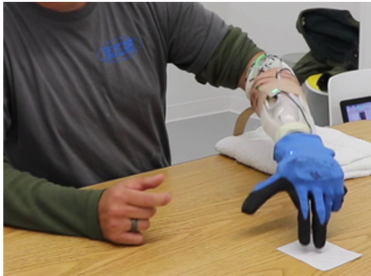
Fig. 1 An amputee subject moving a card with the SoftHand 2 Pro. The index point grasp is used to execute the task
