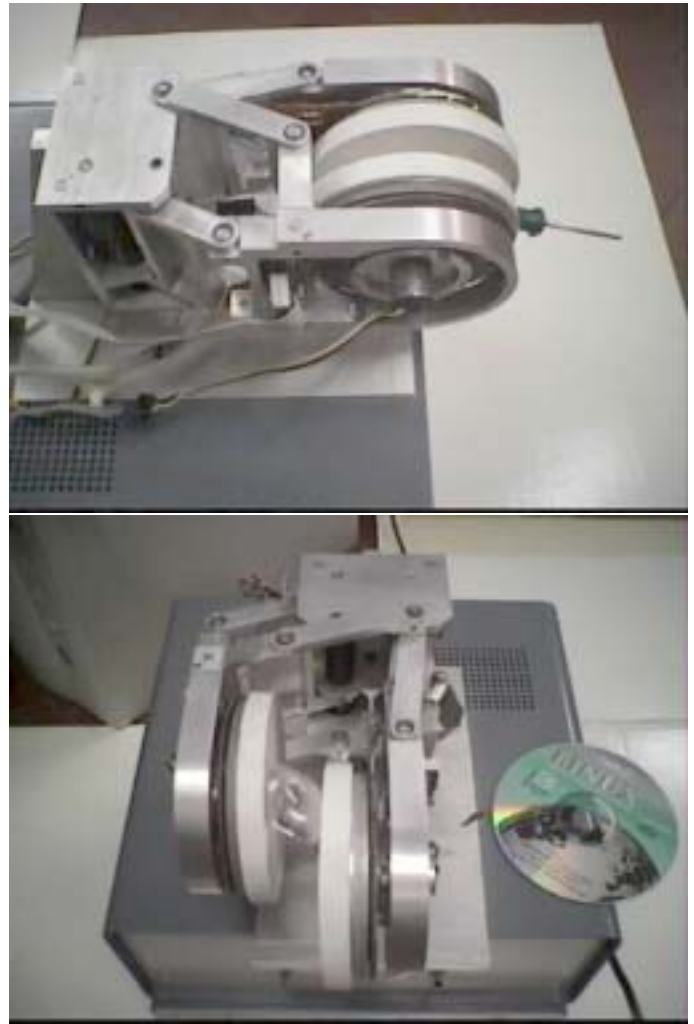
Fig. 14. Photographs of DxGrip-II showing the dimensions and the kinematic arrangement.
