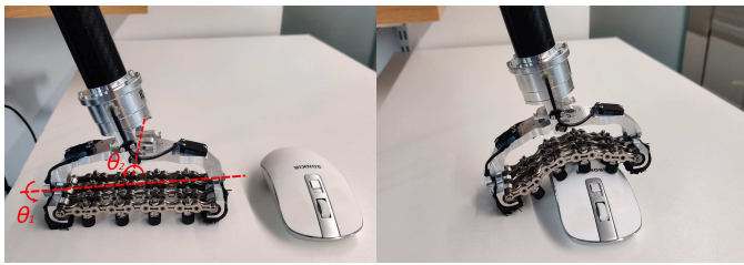
Fig. 11. The SoftFoot-Q, an adaptive foot for quadrupeds. \theta_1 and \theta_2 indicate the passive joints of the ankle.
