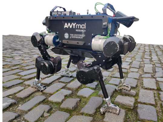
Fig. 1. ANYmal with adaptive feet stepping on rough terrain.
