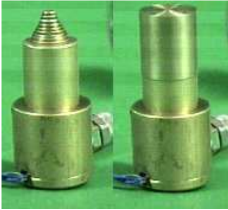
Figure 3: The prototype CASR display on the left and appearance of the kinesthetic display used in the experiments on the right.
