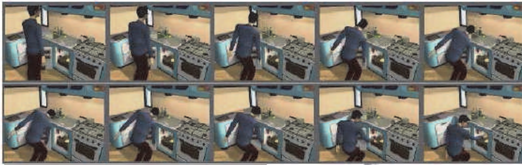
A motion computed by a planning algorithm, for a digital actor to reach into a refrigerator
