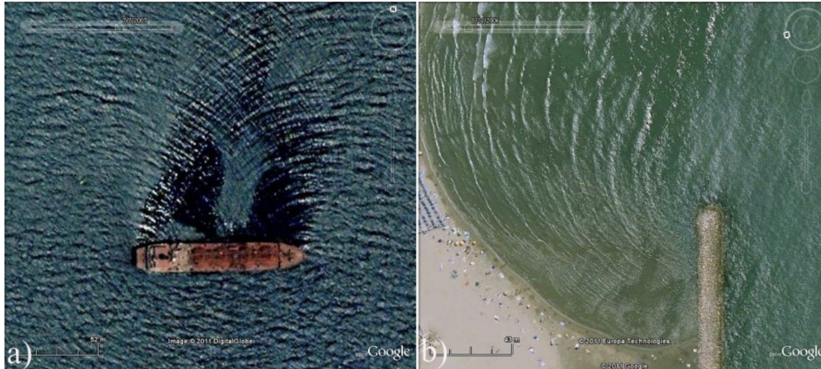
Figure 2: a) Diffraction produced by a boat: Cyprus, 7/7/2007, coordinates: 34^{\circ} 56' 27.21'' N , 33^{\circ} 39' 17.36'' E . b) Diffraction of waves against the end of a protection barrier: La Grande-Motte, France, 8/21/2006, coordinates: 43^{\circ} 33' 18.71'' N , 4^{\circ} 05' 20.01'' E .
