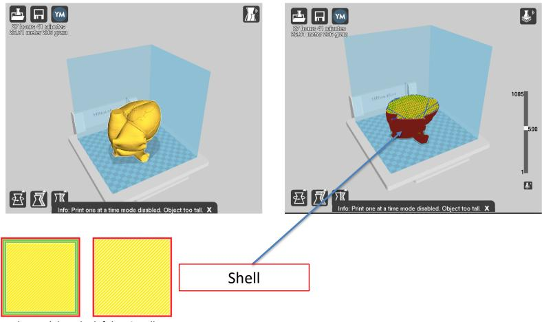
The model on the left has 3 walls, the model on the right has a single wall.
