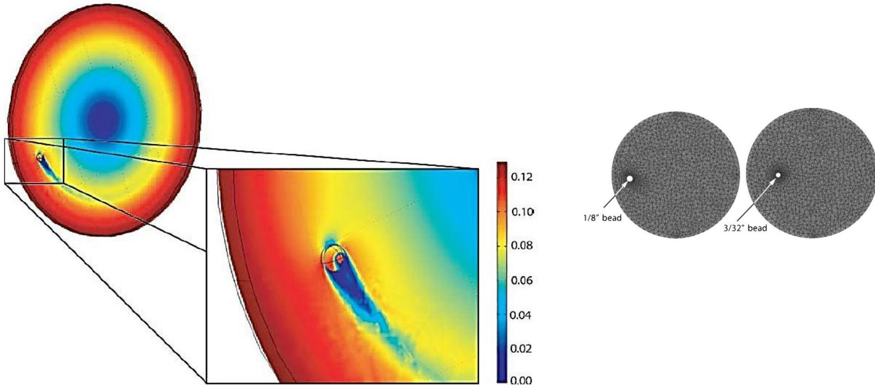
FIG. 3. Fluid velocity distribution in the bioreactor. The velocity (measured in m/s) increases with radius from the center of the bioreactor except in the region near the spherical bead (see inset). The disruption in the velocity field is responsible for the elevated shear stresses in the fluid.
