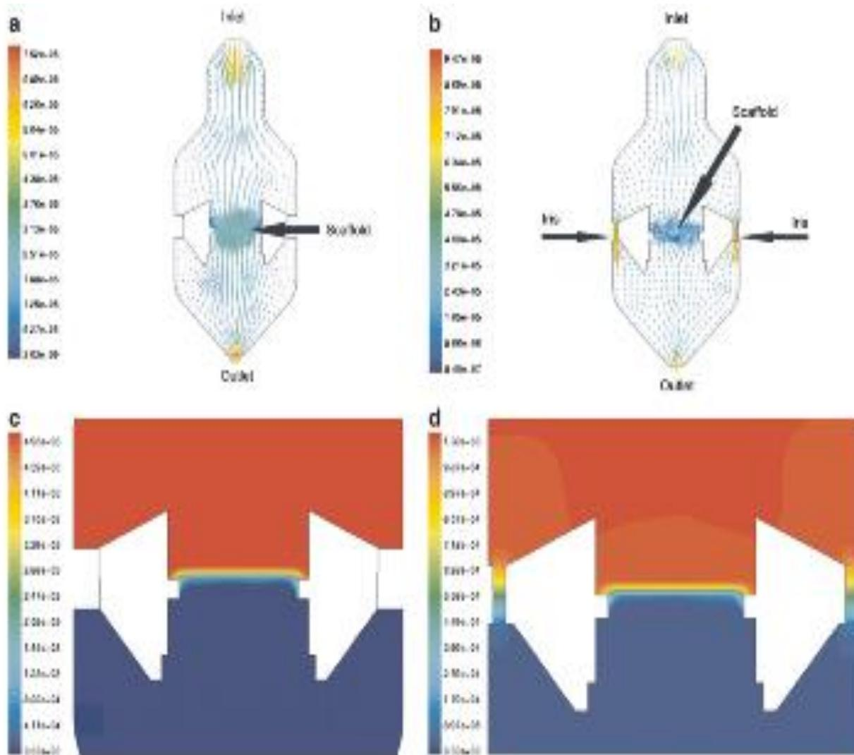
Laminar flow bioreactor for **primary human mesenchymal stem cells** [1].
