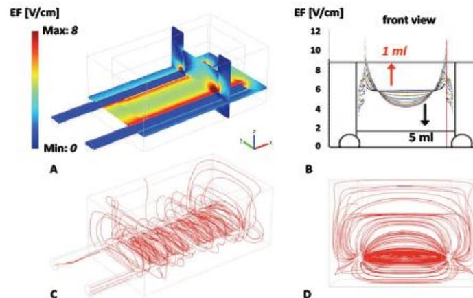
Fig. 3. Distribution of the EF within the culture chamber: contours of the EF magnitude (A) and EF streamlines distribution (C, D) with a 8-V amplitude square voltage input; (B) EF magnitude and distribution evaluated at different medium volumes within the chamber.
