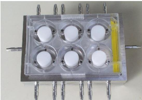
The **TransMIT Pressure system** is projected for cultivation and pressure stimulation of cell-matrix-composites. A special aspect of this bioreactor is that the device is composed in a way that generally available tissue culture plates (with up to 96 cavities) can be used as part of the new bioreactors. The stimulation of the cells or composites can be done with defined or undefined pressure. The durability and frequency of the pressure stimulation are freely programmable by user.
