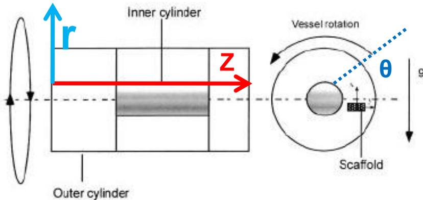
Figure 1. Sketch of the rotating bioreactor (on-ground conditions).
