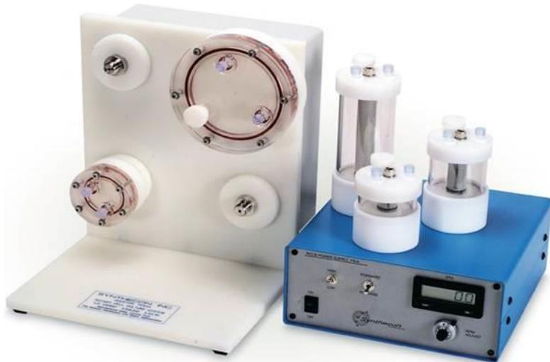
The **Rotary Cell Culture System (RCCS)** is a unique cell culture technology for culturing both suspension and anchorage-dependent cells. It is the first bioreactor system designed to simultaneously integrate the ability to co-culture cells, and the features of low shear force (and consequently low turbulence), and high mass transfer of nutrients. Together these properties encourage spheroid formation and proliferation of cells within the three-dimension spheroids.
