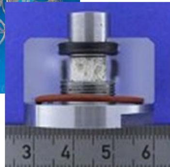
The **Zetos System** is a novel 3D Bioreactor (Zetos™) capable of maintaining human bone biopsies in a viable and responsive state for up to 45 days.
