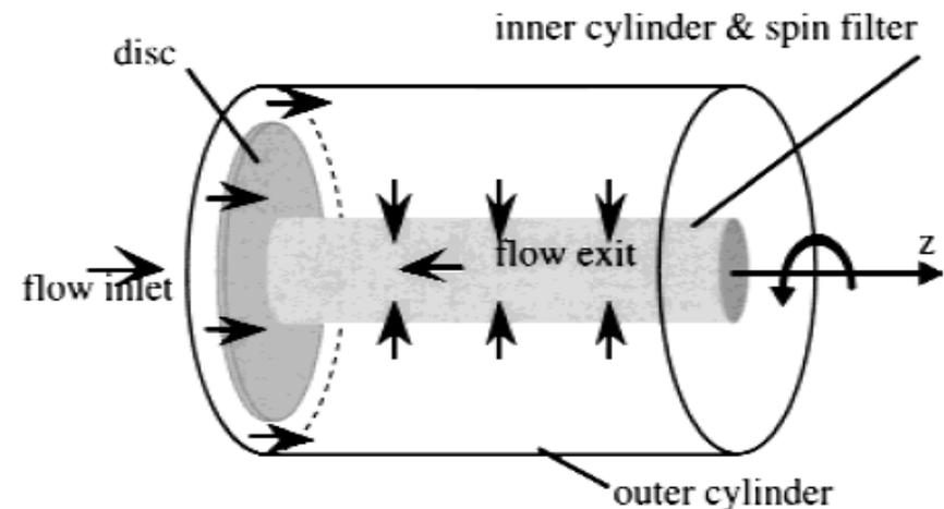
Figure 1. Rotating-wall perfused-vessel geometry.
