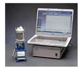
**CartiGen Bioreactor** apply an oscillatory compressive or tensile stimulation to disc shaped samples. A pressurized non-permeable membrane compresses the samples, applying to them a controlled hydrostatic pressure. It integrates a porous platens with the bottom of the chamber to permit perfusion through the sample constructs, to allows the direct flow through the construct while applying oscillatory compressive stimulation.
