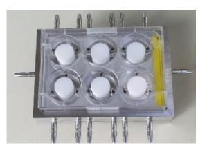
The **TransMIT Pressure system** is projected for cultivation and pressure stimulation of cell-matrix-composites. A special aspect of this bioreactor is that the device is composed in a way that generally available tissue culture plates (with up to 96 cavities) can be used as part of the new bioreactors. The stimulation of the cells or composites can be done with defined or undefined pressure. The durability and frequency of the pressure stimulation are freely programmable by user.
