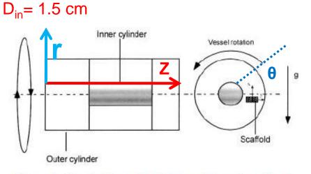
Figure 1. Sketch of the rotating bioreactor (on-ground conditions).
