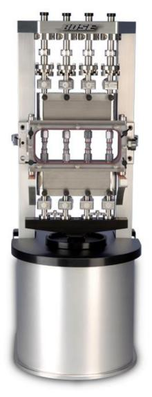
**Bose Corporation** has developed a multi-specimen **ElectroForce® BioDynamic®** test instrument for intervertebral disc and other orthopaedic applications to mimic the complex loading that tissues experience in vivo. Spinal discs, cartilage and bone tissues, scaffolds and tissue-engineered constructs can be characterized under multiaxial stimulation.
