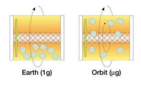
The rotating-wall perfused-vessel (RWPV) bioreactor, used for both **microgravity** and **Earth-based** cell science experiments, is characterized in terms of the fluid dynamic and fluid shear stress environment.
