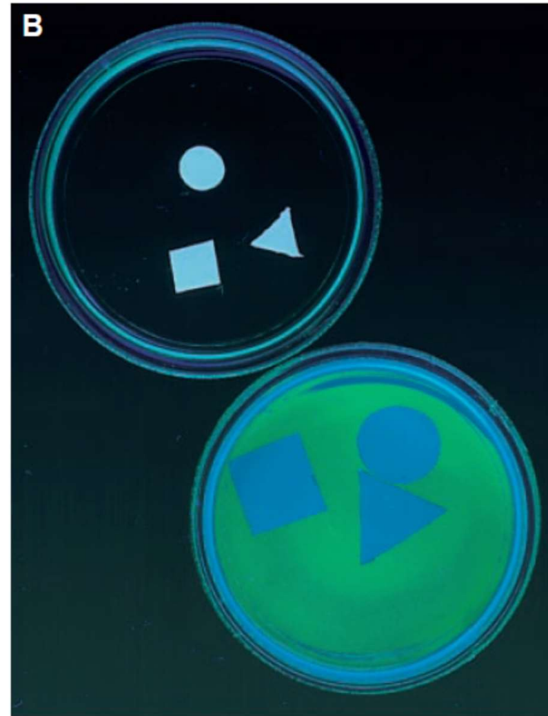
Fig. 2. (A) The adsorption of pyranine-3 per MAPTAC monomer as a function of pyranine-3 concentration in the swollen state at 25°C and in the shrunken state at 55°C. The MAPTAC concentration was 30 mM. (B) The shrunken gels at 55°C (upper dish) and the swollen gels at 25°C (lower dish) under illumination with UV. In the shrunken state, the gel adsorbed all of the pyranine molecules, but in the swollen state, the gel released them all as seen by their fluorescence. [Photograph by Felice Frankel, © 1999]
