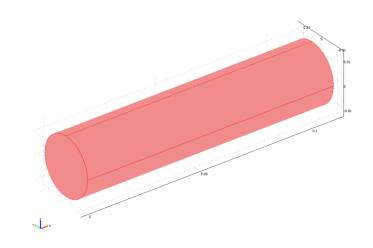
D = 25 mm L = 110 mm  $Q_{in} = 5 L/min$
