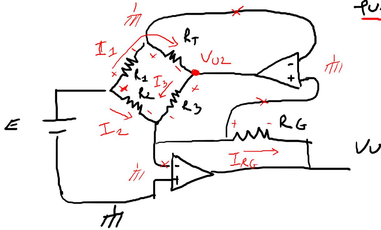
$$V_u = -R_G I_{RG} \quad I_{RG} = I_3 + I_2$$
