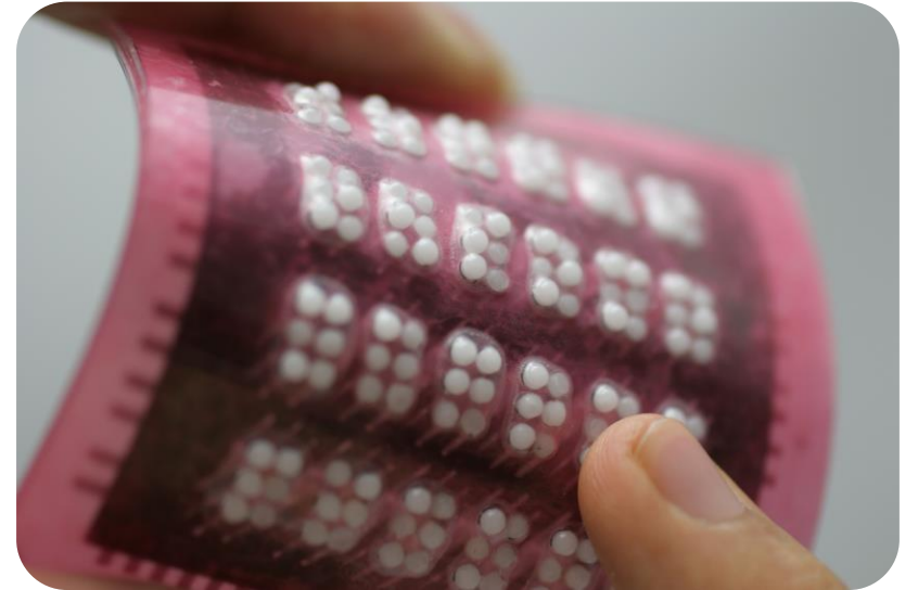
Braille display from the University of Tokyo
