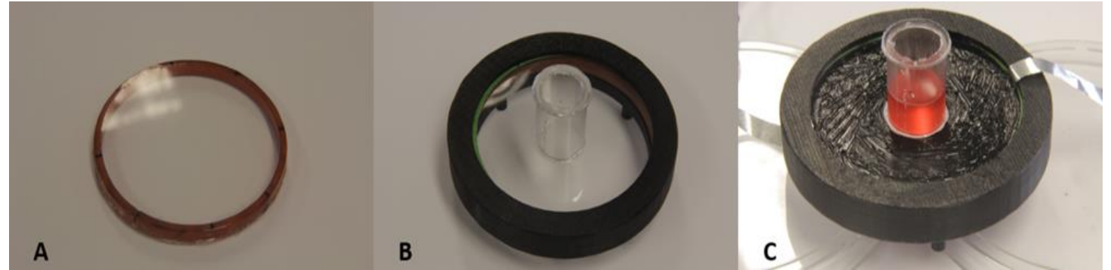
The bioreactor at various stages of fabrication: A) the membrane, B) the flexible central well, C) the complete bioreactor mounted within its case, containing the cultured cells and 1 mL of medium within the well and equipped with the carbon grease electrodes.
