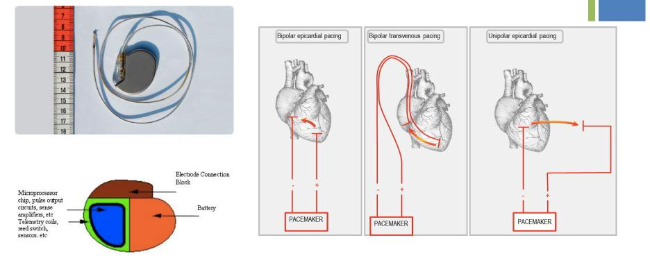
Sensing (and pacing) is accomplished with one of two configurations, bipolar and unipolar. In bipolar, the anode and cathode are close together, with the anode at the tip of the lead and the cathode a ring electrode about 2 cm proximal to the tip. In unipolar, the anode and cathode may be 5–10 cm apart. The anode is at the lead tip and the cathode is the pulse generator itself (usually located in the pectoral region).
