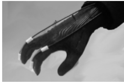
Fig. 17. Sensing glove and the electrogoniometers for the calibration phase.
