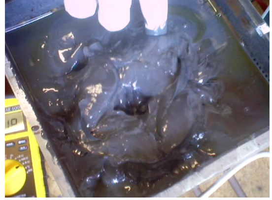
Fig. 23. Picture of the hollow square-shaped object, obtained inside the MR fluid.
